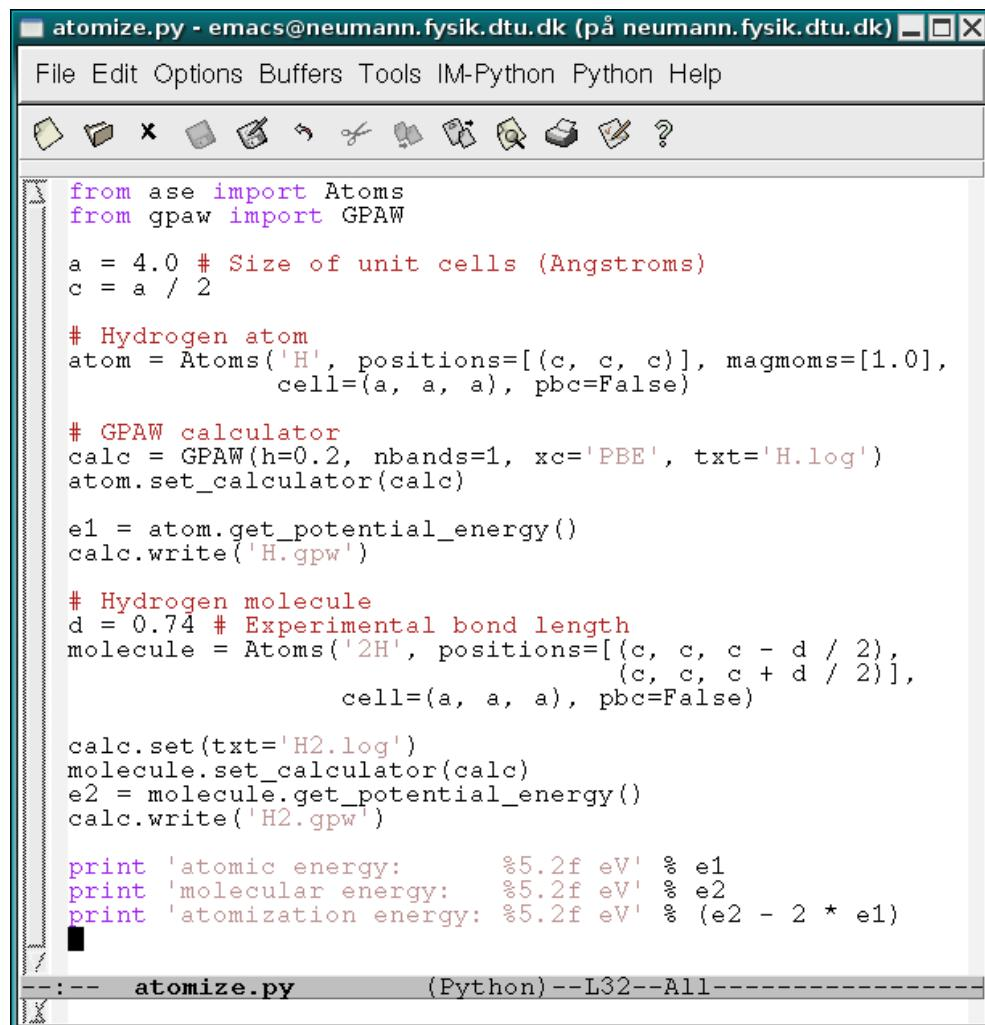
The screenshot shows an Emacs window titled "atomize.py - emacs@neumann.fysik.dtu.dk (på neumann.fysik.dtu.dk)". The window contains Python code for calculating the atomization energy of a H<sub>2</sub> molecule using the ase and GPAW libraries. The code defines unit cells for hydrogen atoms and molecules, performs calculations, and prints the atomic, molecular, and atomization energies.
