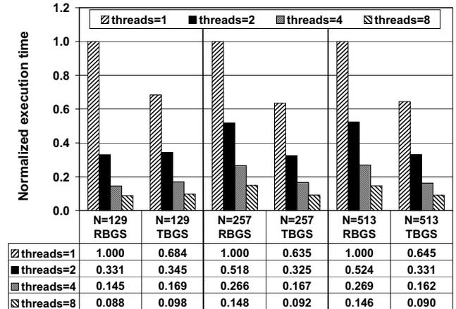
Figure 12: Normalized execution time of the parallel multigrid solvers with RBGS- and TBGS-smoothers for  $N=129$ ,  $N=257$  and  $N=513$  on the 8-way CMP/SMP UltraSPARC IV+ system. The execution time is normalized relative the single processor RBGS multigrid solver.
