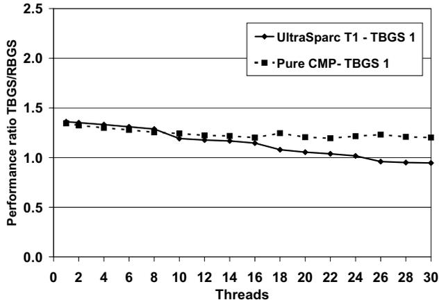
**Figure 8: Performance ratio per step between TBGS and RBGS for the 32-way UltraSPARC T1 and the simulated 32-way pure CMP,  $N=129$ .**
