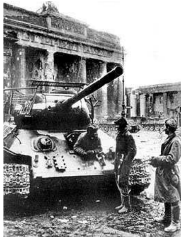
Figure 10.1: Soviet T-34 tank with wire mesh for protection against the Panzerfaust anti-tank weapon.[?]
