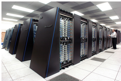
Figure: BlueGene/P supercomputer. Our largest calculations use 32768 or 65536 CPUs (Source: Flickr, by “Argonne National Laboratory”).
