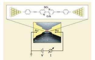
A molecular switch is a molecule connected between two conducting electrodes. The molecule can switch between two different states with high and low electrical conductance.<sup>1</sup>
